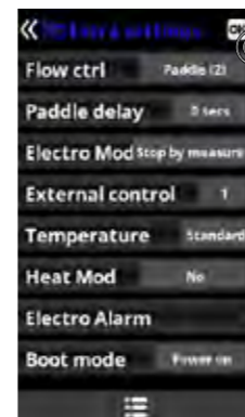
Go to the Flow ctrl menu and select Paddle (2). Press OK to confirm the selection. By default, the box is set to Paddle or gas (3).
