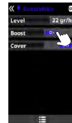
Shock treatment: Continuous filtration for 24 hours at maximum intensity. Automatic return to the programmed filtration mode. During the shock treatment, ORP control can be deactivated.
