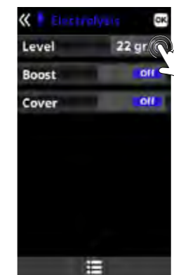
Level: Production of chlorine (g/h) desired for electrolysis. Production of chlorine (%) desired for hydrolysis.
