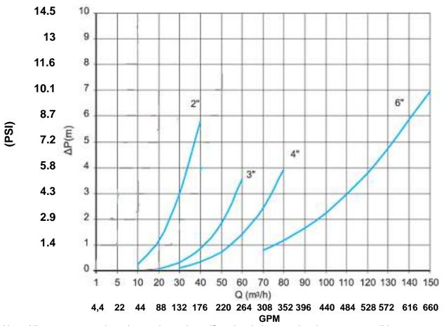
Note: All measurements have been taken using orifice size d=4mm, under clean water conditions.
