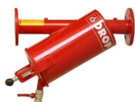
The filter is cleaned manually, by means of opening the drain vane at the lid, during the irrigation proccess, or for finer cleaning, the inner cartridge should be dissasembled and washed with water.
