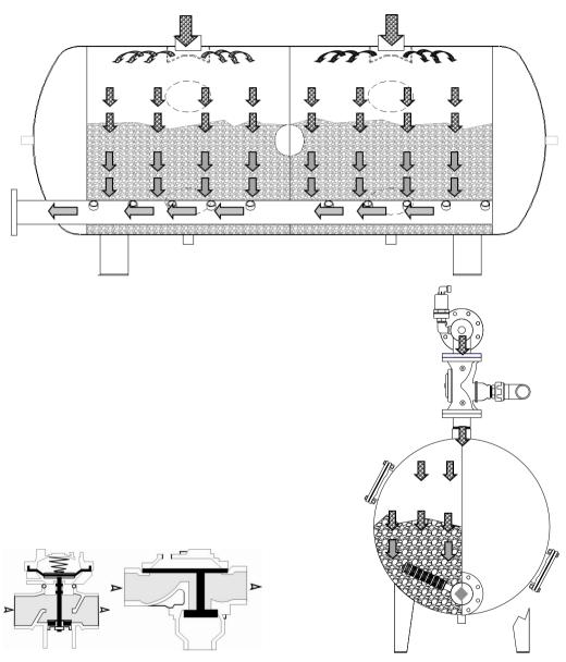
During filtration the water passes through the inlet collector, through the backflush valves and get into the chambers of sand media filter from the top of it.
