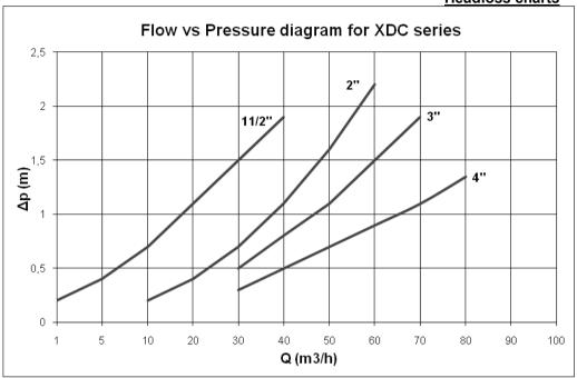
Note: All the measurements have been taken with media size 1.2-2.4mm, in clean water conditions.
