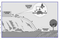
• In any case, whenever the installation does not allow to maintain necessary the sufficient pressure for the backwash one, it is advisable to place a manual valve when coming out (of butterfly), regulated properly to stabilize the pressure.
