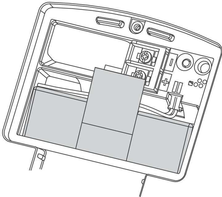
**EN** Place the battery in the battery storage area. Close the battery compartment and secure with the screw.
