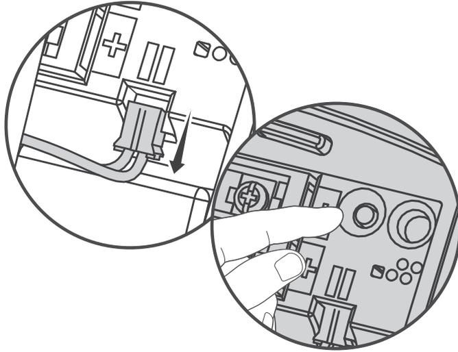
**EN** The reset button is located in the battery compartment. If it's necessary to reset the repeater:
