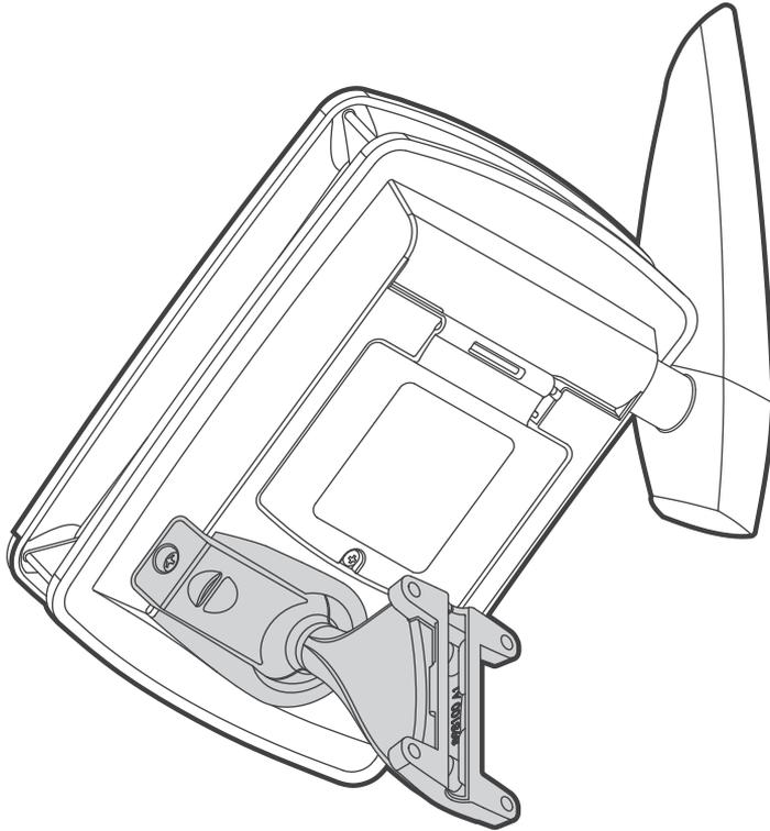
**EN** Choose the necessary mounting hardware. The swivel ball mount has screw holes for wall mounting as well as slots for using stainless steel band clamps (approximately  $\frac{5}{8}$ " or 15.8 mm wide).
