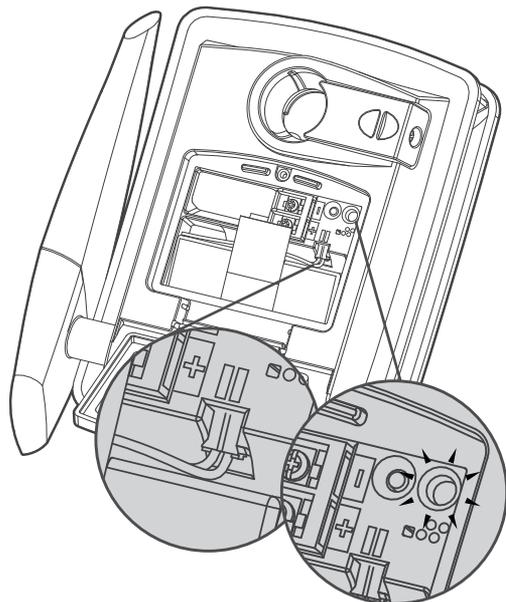
**EN** Open the battery compartment using a small screwdriver.
