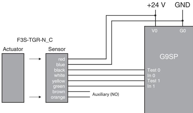
**Series connection Application, up to 3 Sensors with G9SP**
