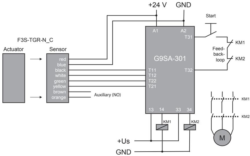
**Series connection Application, up to 3 Sensors with G9SA-301**
