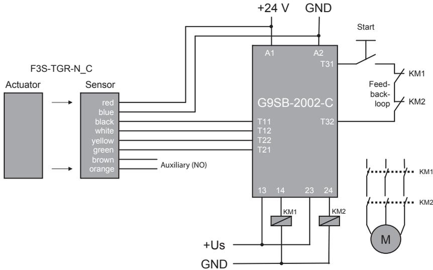
Series connection Application, up to 3 Sensors with G9SB-2002-C
